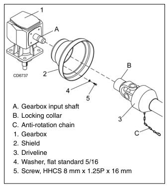
Figure 30. Driveshaft Installation
